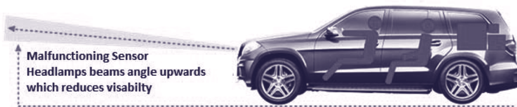
Fig. 1. Headlamp beam movement due to different loading conditions
