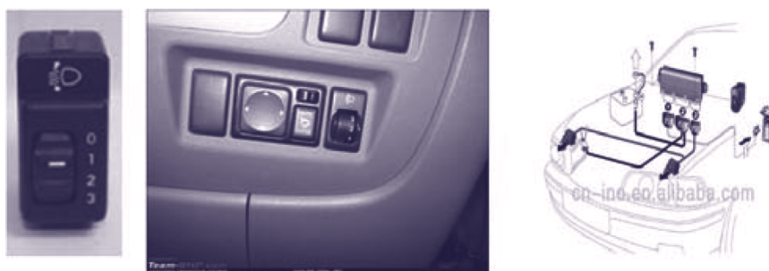
Fig. 2. Manual headlamp leveling switch near the driver
